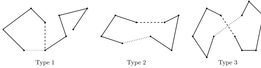
45 **Figure 1.** The three types of flips in plane spanning paths.
