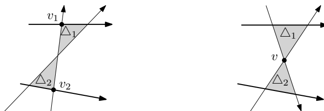
Figure 7: Left: the two triangular cells \Delta_1 and \Delta_2 do not form an hourglass, because they share a vertex that is not an exit vertex. Right: the two triangular cells \Delta_1 and \Delta_2 form an hourglass because they share an exit vertex.
