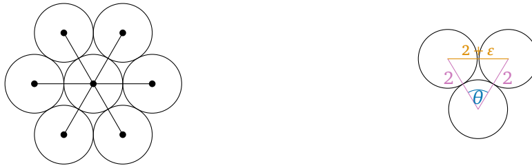
(a) The 6-star has only this unique weak UDCR. (b) Looking at two neighboring leaf disks around the center disks. If \epsilon = 0 then \theta = \frac{\pi}{3} but setting \epsilon > 0 implies \theta > \frac{\pi}{3} . Then six disks cannot be placed around the center disk.
