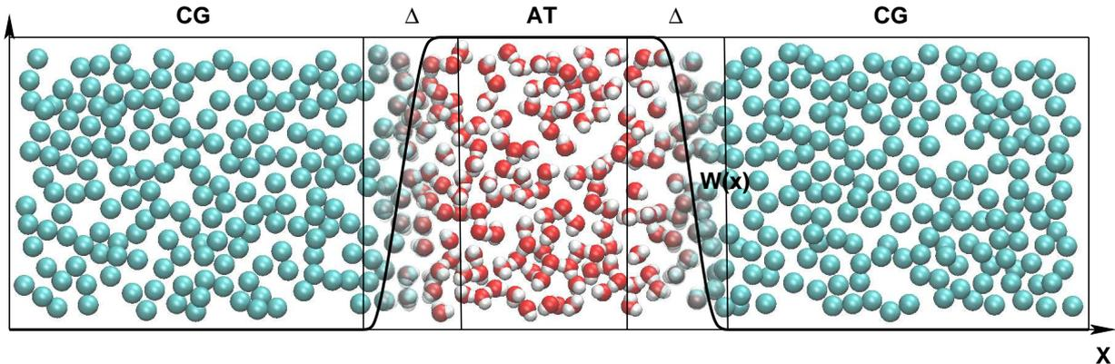
FIG. 1. A schematic representation of liquid water in AdResS. CG indicates the region at coarse-grained resolution, AT that at atomistic resolution, and finally  $\Delta$  the transition region where molecules change resolution according to a smooth switching function  $w(x)$ .
