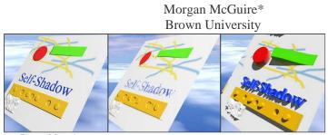
*Bump Mapping Parallax Mapping Steep Parallax Mapping* **Fig. 1** A <u>single</u> polygon with a high-frequency bump map.
