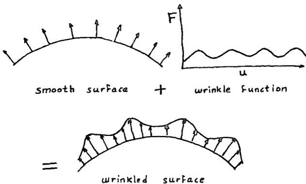
Figure 2 - Mapping Bump Function
