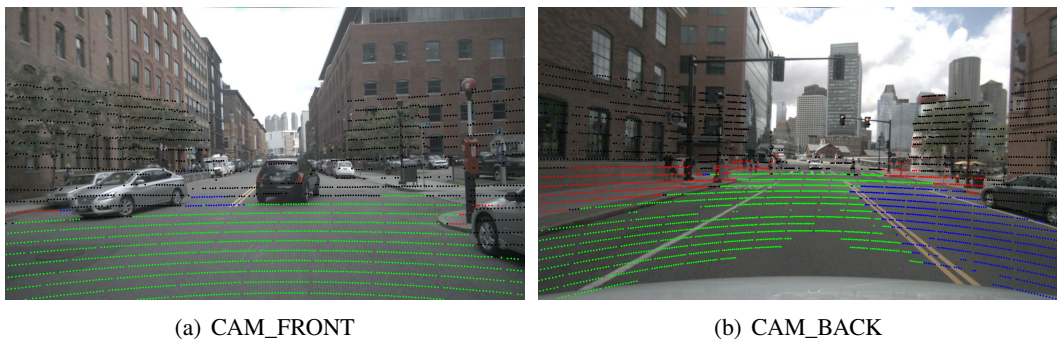
Figure 6.15: Projection of LiDAR point cloud in camera image (scene-0103).
