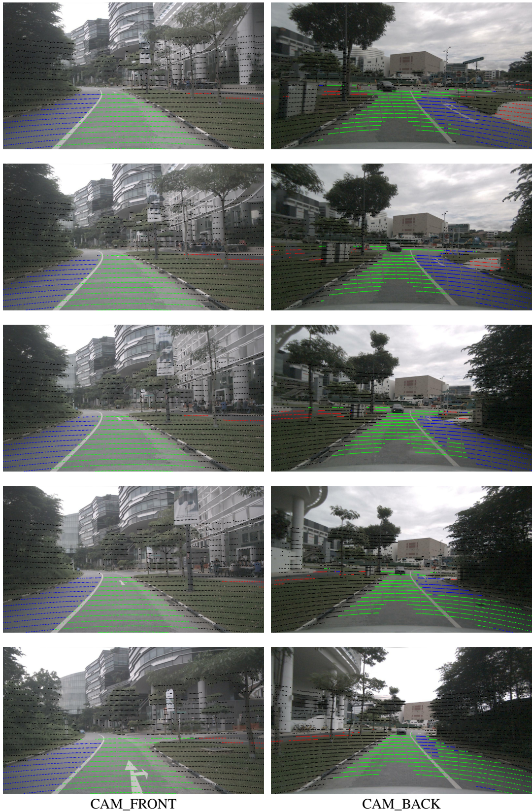
Figure A.17: Projection of LiDAR point cloud in camera front- and back-view perspective. Providing sequence of scene samples (scene-0269). False detection mostly appears in back-view images, whereas front-view mostly remains stable.
