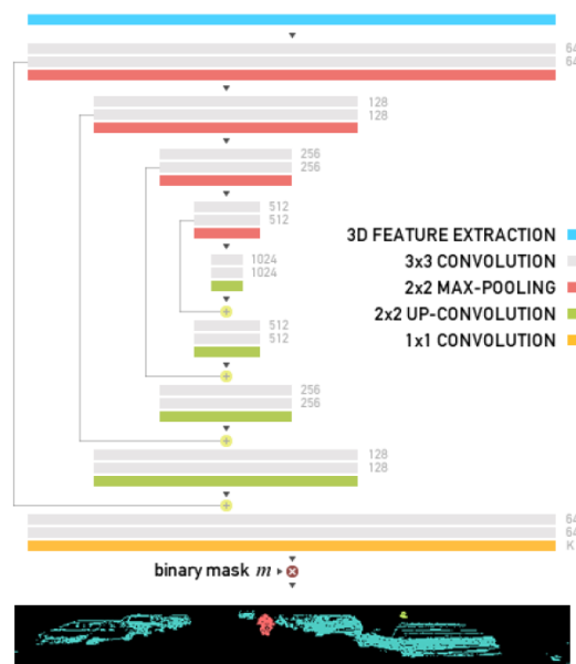
Figure 4.11: Architecture of proposed LU-Net as backbone architecture containing processed segmentation mask [3, 41].
