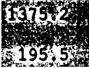
Fig. 8. First experiment, binarization by Otsus method.
