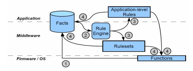
*Figure 1*: Component diagram of FACTS architecture: Low-level events start execution by creation of new facts (1), which trigger the rule engine (2) to match rules against fact repository (3) and eventually fires rules (4).
