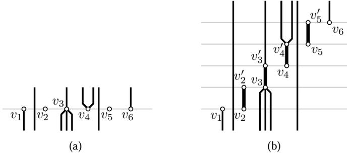
Fig. 12. **(a)** A level  $V_i$  with width  $\lambda_i > 2$ . **(b)** In order to reduce the level-width, we replace  $V_i$  with  $\lambda_i - 1$  levels. Thick edges are the stretch edges.
