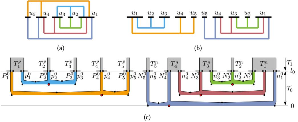
Fig. 8. **(a)** Representation  $\mathcal{R}$  of  $\varphi$  with negative clauses  $(\bar{u}_1 \vee \bar{u}_4 \vee \bar{u}_5)$ ,  $(\bar{u}_1 \vee \bar{u}_3 \vee \bar{u}_4)$  and  $(\bar{u}_1 \vee \bar{u}_2 \vee \bar{u}_3)$  and positive clauses  $(u_1 \vee u_4 \vee u_5)$  and  $(u_1 \vee u_2 \vee u_3)$  and **(b)** its modified version  $\mathcal{R}'$  in Lemma 4.1. **(c)** Tier  $\mathcal{T}_0$ .
