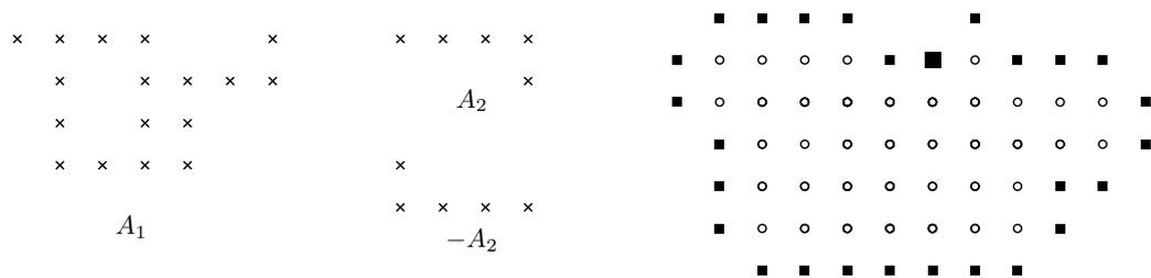
■ **Figure 9** The sets  $A_1$  and  $A_2$  of cell centers of the polyominoes  $P_1$  and  $P_2$ , respectively, from Figure 1, the Minkowski difference  $F = A_1 \oplus (-A_2)$  (circles), and the set of valid composition vectors (squares).  $P_1$  and  $P_2$  have 27 compositions. The composition from Figure 1 is highlighted.
