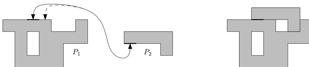
■ **Figure 1** Aligning the edges connected by the arrow-curve creates a composition of the two polyominoes  $P_1$  and  $P_2$ , as shown on the right. The alignment along the dotted curve does not create a valid composition because it would lead to an overlap between  $P_1$  and  $P_2$ .
