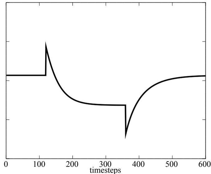
Figure 1: The friction coefficient under simulated velocity stepping
