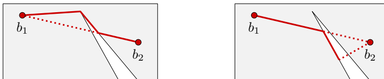
Figure 1: Attraction is not symmetric. In this two-dimensional example b_1 attracts b_2 (left) but b_2 does not attract b_1 (right).
