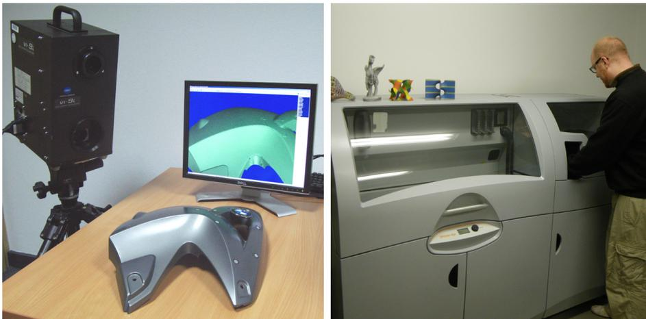
**Figure 1.1:** A 3D Scanner and a 3D printer. Picture taken from [Pro].
