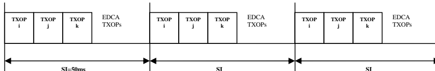
Fig. 2. TXOP distribution for three streams named as i,j and k
