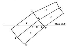
Fig. 4. Gouraud shading, applied to approximated cone of Fig. 1.
