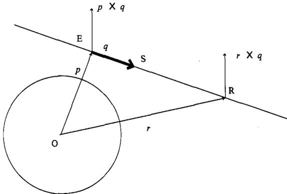
Figure 8. Geometry for computation of ray projection
