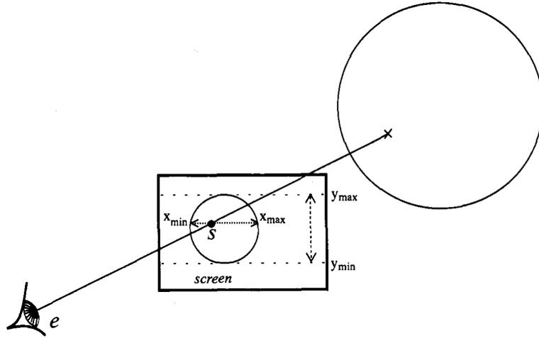
Figure 17. Geometry for scan-line and y-bounds calculations
